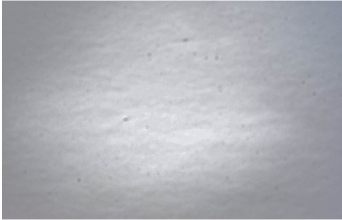
Fig. 8: Dust spots on the sensor made visible: this sensor badly needs cleaning.
