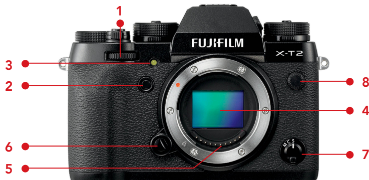
Fig. 1: X-T2 frontal view: front command dial with integrated button (1), Fn button (2), AF assist lamp/self-timer indicator lamp (3), X-Trans sensor (4), electronic lens contacts (5), lens release button (6), focus selector (7), flash sync connector (8)
