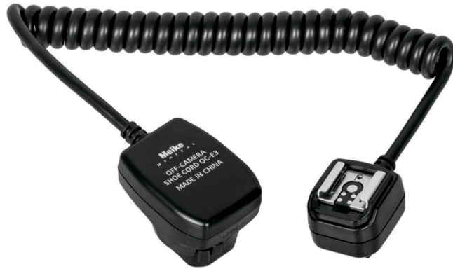
Fig. 19: A Canon-compatible TTL extension cord works with the X-T2. However, since the extra power line for Fuji's tiny EF-X8 flash unit isn't looped through, this flash can only be used directly on the camera's hot-shoe mount.
