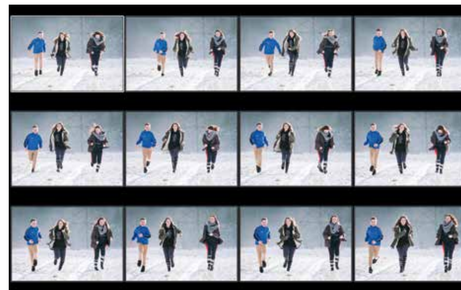
Fig. 44: AF tracking with AF-C and burst mode: The predictive autofocus was tracking one of the kids with the selected AF zone while they were running toward the camera. To make this kind of shot work, it's vital to follow the subject with the active AF frame or AF zone, making sure it's always covering the part of the subject that is supposed to be in focus.
