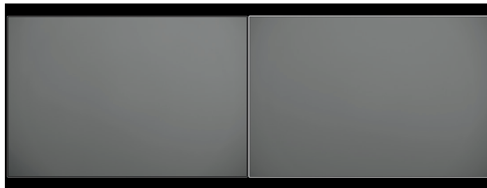
Fig. 20: This illustration shows a black sheet of paper and a white sheet of paper. Both were photographed with the camera's spot metering without any exposure correction. As you can see, the camera delivered a middle-gray exposure in both cases. In order to get an image that reflects the actual brightness of the subject, the metered exposure has to be adjusted.
