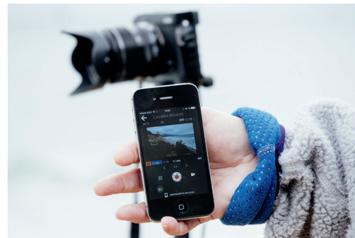
Fig. 73: Camera Remote offers a simple interface to control your camera with a smartphone or tablet. To autofocus, double-tap on a specific part of the WYSIWYG live view and wait for the green confirmation rectangle to appear. Sadly, there is no live histogram, and you can't magnify the live view. There is a rudimentary shooting menu, a virtual shutter button, and a playback button that allows you to review images and transfer JPEGs to your mobile device.
