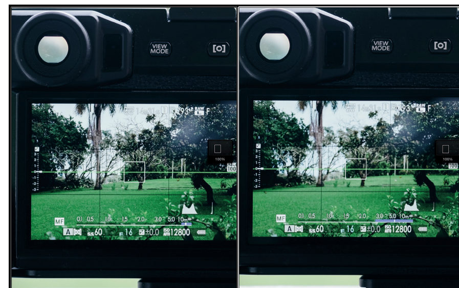
Fig. 37: Setting the hyperfocal distance with the electronic distance and DOF scale: instead of focusing on a predetermined distance, manually change the focus distance until the blue DOF bar touches the infinity mark on the right end of the scale. This gives us the hyperfocal distance for a given aperture and focal length. This image shows the hyperfocal distance for a XF35mmF2 lens at f/16 and both the PIXEL BASIS format (left) and FILM FORMAT BASIS format (right).
