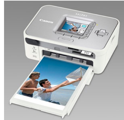
Figure 1-9: Canon SELPHY CP750 dye-sublimation printer, 300 dpi, print-size up to 10 x 20 cm, (Courtesy Canon Germany)
