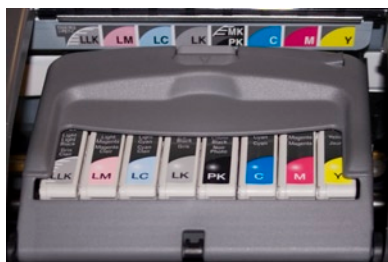
Figure 1-16: Though the Epson R2400 may use 9 different inks, only 8 cartridges may be in place at any point of time. You may either have either 'Photo Black' (PK) or 'Matte Black' (MK) in place.
