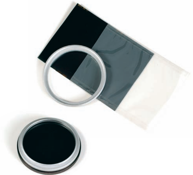
▲ The photographic results using unexposed slide film as a filter are similar to those using an RG715, except for the reduced image sharpness.
