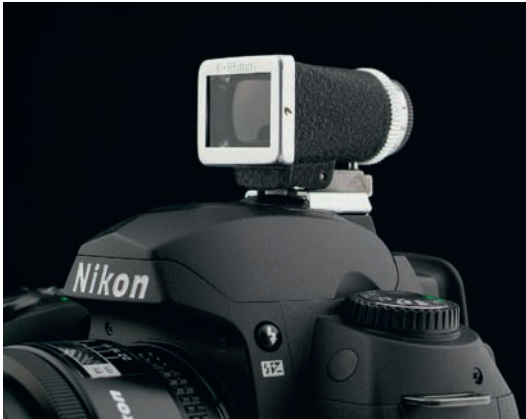
▲ With SLR cameras, an attachable, external viewfinder makes it possible to frame the picture even with an infrared filter attached to the main lens.
